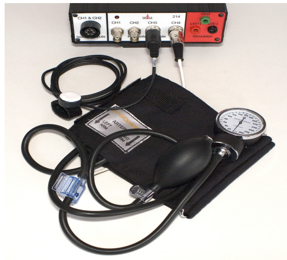
Figure HP-6-S3: The PT-104 pulse transducer and the BP-600 non-invasive blood pressure transducer connected to an IWX/214.
