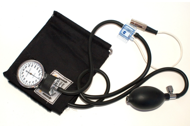
Figure HP-6-S1: The BP-600 non-invasive blood pressure transducer.
